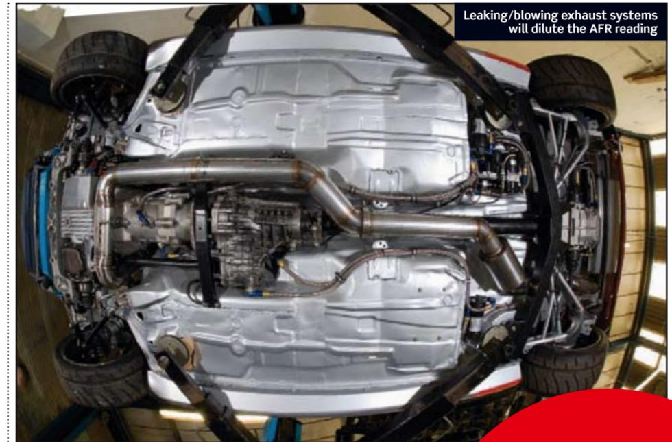
Leaking/blowing exhaust systems will dilute the AFR reading
